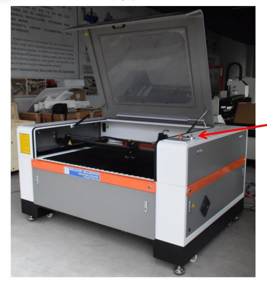
Displays the current triggered by the laser tube, and a knob on the side adjusts the amount of current triggered
